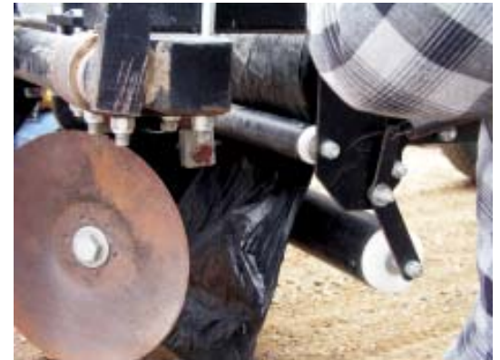
Side view of cradle on plastic mulch applicator.
